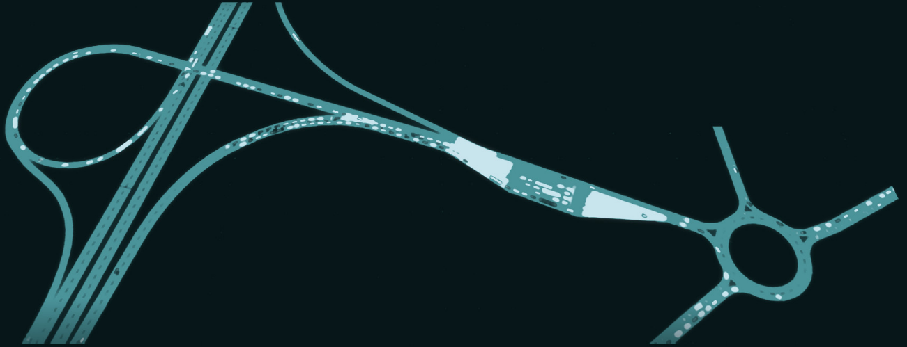
A1 motorway model: microsimulation of the toll plaza and interchange
